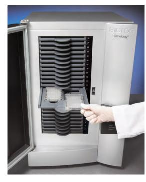
The Biolog OmniLog<sup>®</sup> incubates and monitors 50 microplates, or 1,920 phenotypic assays simultaneously to measure physiological responses in diverse microbial cells.
